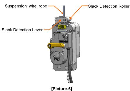
①-1 Push down the Slack Detection Lever and insert the end of the suspension wire rope into the BISOLOCK wire rope inlet approximately 16 in (approximately 40 cm). When inserting the suspension wire rope, pass it through the inside of the Slack Detection Roller. (See Picture-6)
